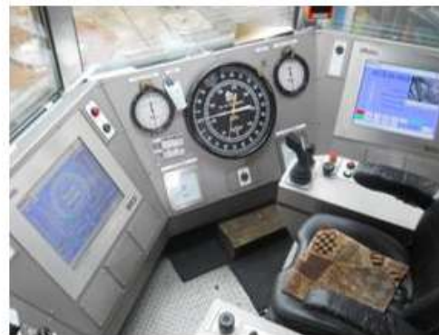
Figure 6. Drilling parameters monitoring boards
