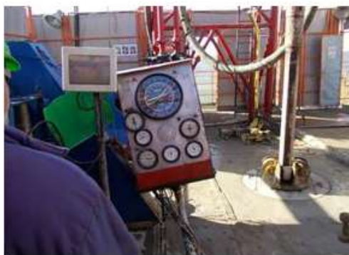
Figure 6. Drilling parameters monitoring boards
