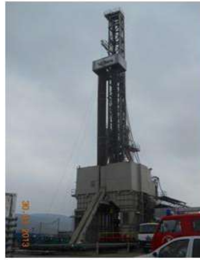
Figure 4. Bentec 350t-AC drilling rig
